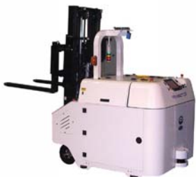
Automatic Trailer Loading Laser Guided Vehicle Load Size: 48"x48" Load Weight: 4,000 lbs Lift Height: 5 feet
