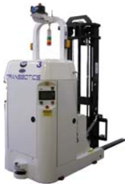
Counter Balance Fork Laser Guided Vehicle Load Size: 48" x 48" Load Weight: 1,800 lbs Lift Height: 5 feet
