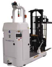
Counter Balance Fork with Load Clamp Laser Guided Vehicle Load Size: 48"x48" Load Weight: 4,000 lbs. Lift Height: 5 feet
