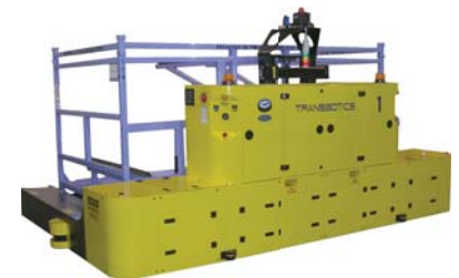
Quad Directional Side Loading Fork Laser Guided Vehicle Load Size: 14'x9' Load Weight: 2,000 lbs Lift Height: 4 feet
