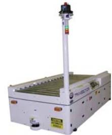
Dual Inline Conveyor Laser Guided Vehicle Load Size: 40" x 48" Load Weight: 2,500 lbs/conveyor
