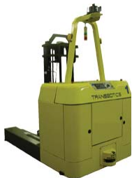
Reach/Lift Fork Laser Guided Vehicle Load Size: 48" X 48" Load Weight: 2,500 lbs. Lift Height: 8.5 feet
