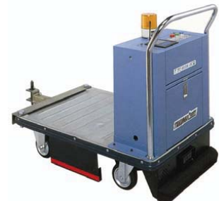
Smart Tugger Tape Guided Cart Load Weight Capacity: 440 lbs
