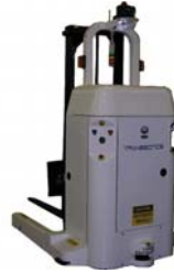
Narrow Straddle Fork Laser Guided Vehicle Load Size: 42" x 48" Load Weight: 4,000 lbs Lift Height: 5 feet
