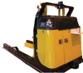
Roll Handling Fork Spreader Laser Guided Vehicle Load Size: 96" Max Diameter Load Weight: 9,000 lbs Lift Height: 3 feet
