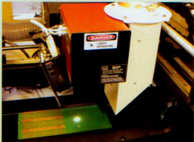
FIGURE 1. Barcode marking and placement are automatic in Conveyor Technologies PCB conveyor system.
